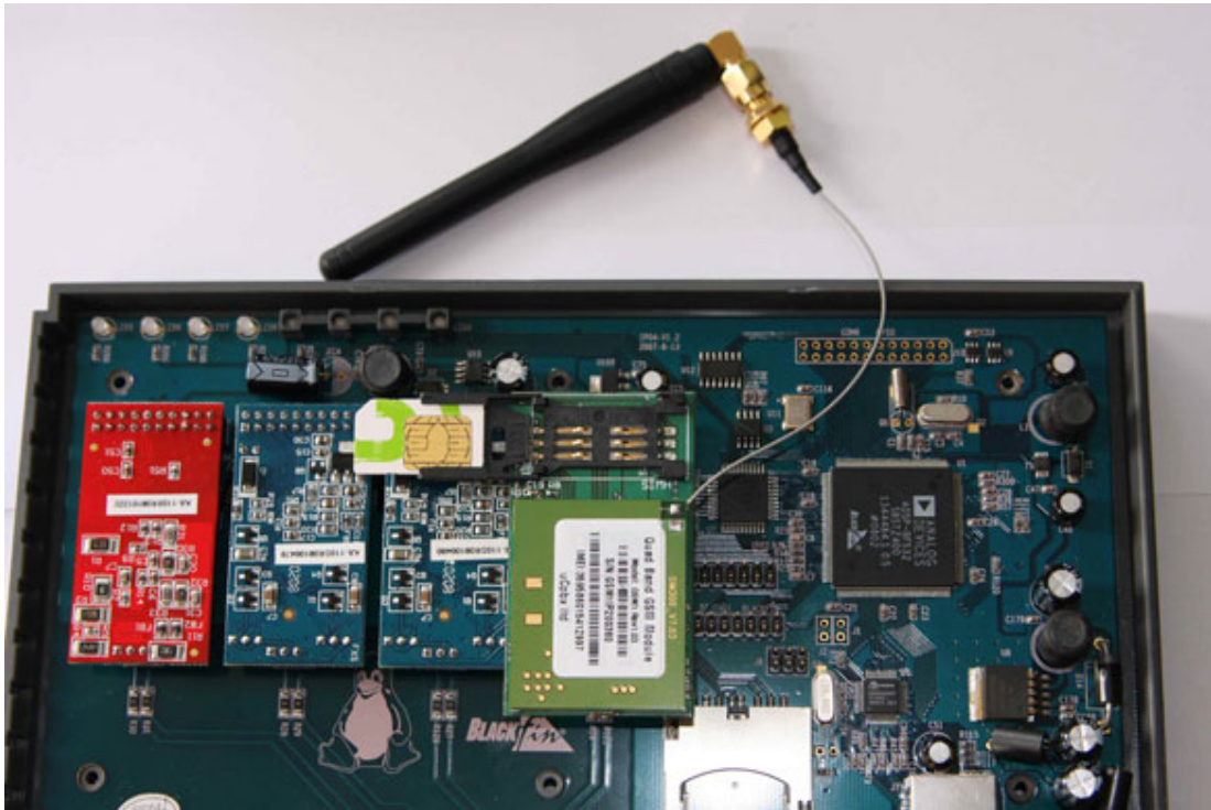
*picture of a IP04 PBX with 1 GSM,1 FXO and 2 FXS modules
